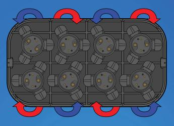
Opposite rotating heads mean the operator does NOT fight the machine.
